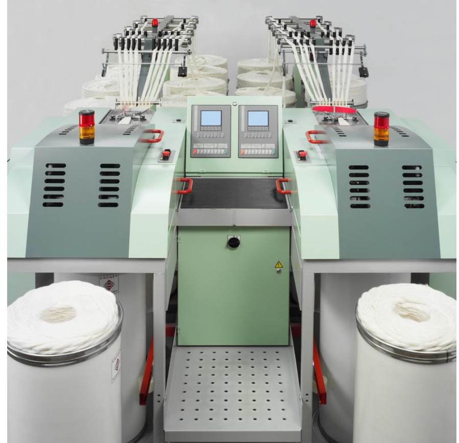
RSB-D 22 Double-Head Autoleveler Draw Frame
