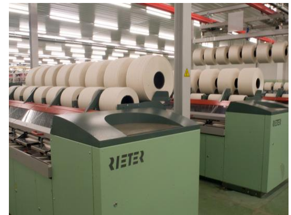
Empty lap removal, full lap loading
